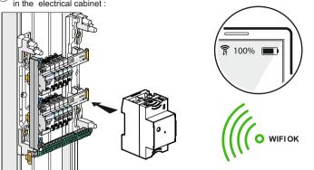
If an internet box is present in the house, check with a smartphone that the Wifi signal level is sufficient. If the signal is not enough, try to bring the internet box to the electrical panel or add a WiFi repeater at the installation.
