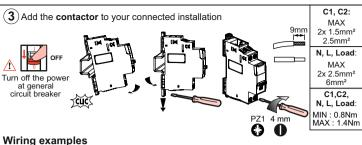
Thanks to its control circuit with integrated power and protection, you no longer need to install a circuit breaker 2A to protect the control circuit if you wire a contact between C1 and C2
