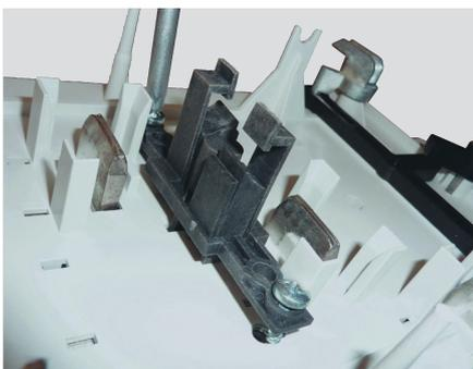
Fix the kit at the rear of the movable part of the support base with the two screws supplied (tightening torque 1 N·m).
