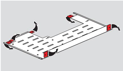
The horizontal insulating plate fixing lugs must be folded back prior to insertion.
