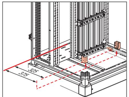
The fixing lugs for the IS chassis rear partitioning are fixed to the enclosure upper and lower crosspieces with a middle screw positioned 375 mm from the front.
