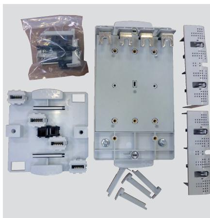
Support bases for DPX<sup>3</sup> consist of a fixed part, a movable part, an anti-withdrawal kit and two terminal shields. They enable screwless connection of a DPX<sup>3</sup> 160 or 250 (when off-load) to the row distribution block with the voltage present.
