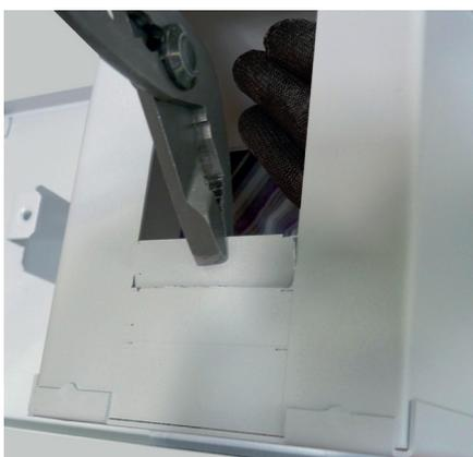
Depending on the circuit breaker used, adjust the size of the window using the specially provided cut-outs.
