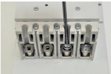
Tighten the upstream and downstream electrical connections using the eight (or six) screws supplied with the circuit breaker. Apply a tightening torque of 7 N·m.
