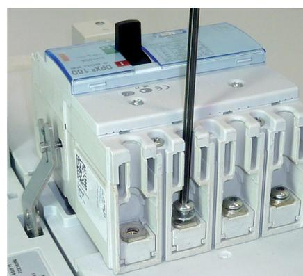
Tighten the upstream electrical connections thanks to the four (for the 4P, 3 for the 3P) screws supplied with the base (tightening torque : 8N m -> DPX<sup>3</sup> 160; 10N m -> DPX<sup>3</sup> 250; 24N m -> DPX<sup>3</sup> 630).
