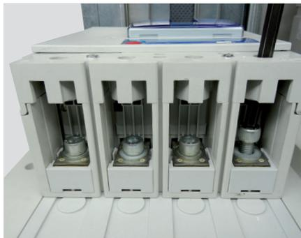
Tighten the upstream and downstream electrical connections using the eight screws supplied with the circuit breaker. Apply a tightening torque of 24 N·m.
