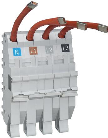
Pre-wired bases require a specific order of operations when mounting DX<sup>3</sup> MCBs. To prevent any risk of contact with live parts, the wires must be connected to the circuit breaker before installing the base on the distribution block.
