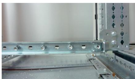
The bottom end support is fixed at the back of the lower part of the functional uprights (use the first two holes).
