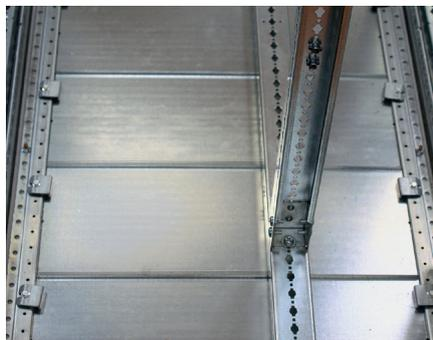
Place the upright and screw it to the fixing lugs using the screws supplied (use the holes on the sides of the upright).
