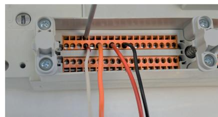
Connect the wires to the module for auxiliary circuits on the movable part of the base. The connection module has screwless terminals and the use of Starfix ferrules is recommended for wiring.
