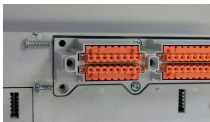
Use six screws for the fixed part, three large ones on the outer edge and three small ones on the inside.
