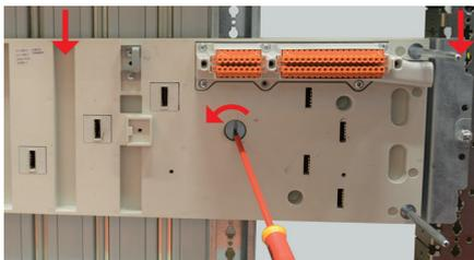
Check that the base is in the correct position by applying gentle downward pressure and then lock the 1/4 turn screw to hold the base in position.
