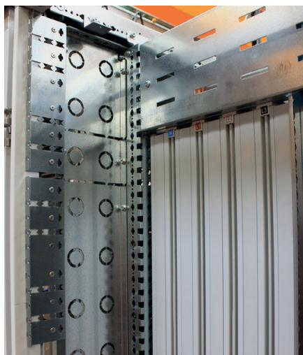
Now simply fix the two front side insulating plates on the column chassis uprights.
