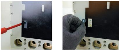
Before mounting the DPX, remove the plate at the back of the product to release the pin. This will trip the circuit breaker whenever the tray (movable part) is no longer in contact with the base (fixed part).
