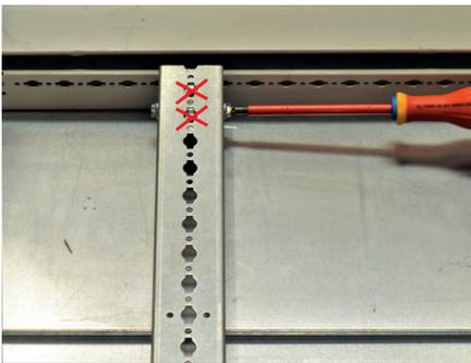
Insert the crosspiece and secure it to the lugs with the screws supplied.
