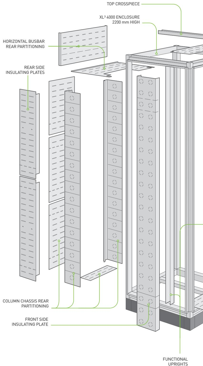
The column chassis consists of all the items used to fix and protect busbars in the enclosure:
