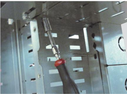
Insert the kit in the side partitioning slot of the chassis, then secure it with the six screws supplied.
