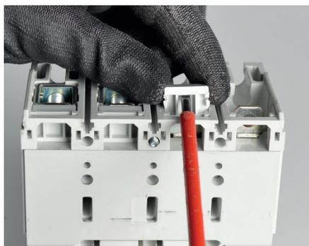
Take out the upstream and downstream rear blanking plates.
