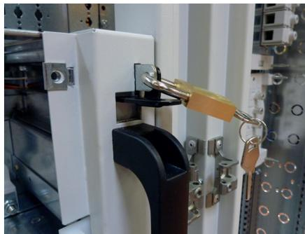
Locking the drawer in each of the three positions is possible with an ordinary padlock maximum diameter 5 mm (for example ref. 4 063 13) inserted at the locking lever. A location is available on each of the two levers.
