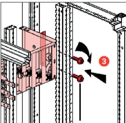
Fix the base to the functional uprights (10 N·m) then to the uprights on the front of the structure using brackets (4 N·m).
