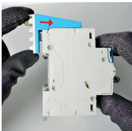
Position the upper part of the connection module (marked "Max 80") on top of the circuit breaker then push it forward to engage the module pin in the MCB. This device ensures correct contact pressure. Do the same for the other poles.
