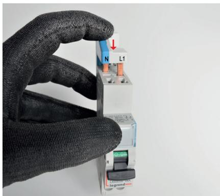
For 1P+N circuit breakers with automatic connection terminals, installation of the connection module is done without tools, the connection module is installed by pressing down.
