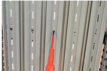
The strips are finally secured with four rows of five screws fixed on the flanges (tightening torque: 1 N·m).
