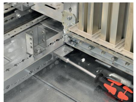
Also fix the four brackets for the top and bottom cover plates 325 mm from the front.
