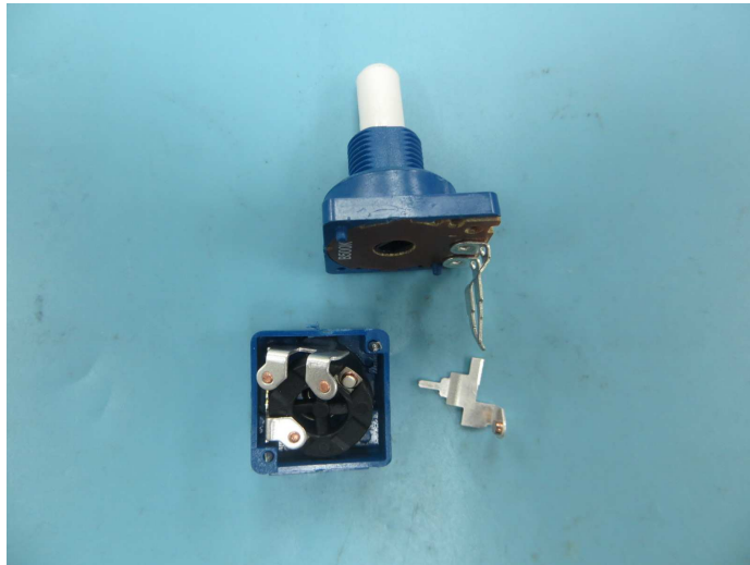
Open view of potentiometer
