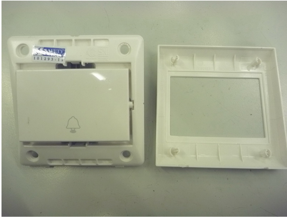
Photo 7: Internal view 1 of model 617011 and 617011E
