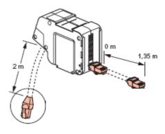
Cable 1.7x8mm in lenght of 1.35m
