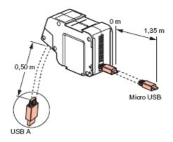
Cable 1.7x8mm in lenght of. 1.35m + plug USB micro B
