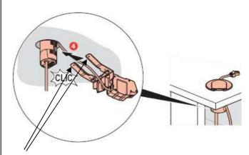
Note: you can install screws to avoid the stealing.
