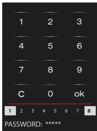
Icons 1 to 8 shown below (only found in the system arming page), indicate the statuses of the zones. In the examples, the zone 1 and 8 are active, while the zones from 2 to 7 are shut off.
