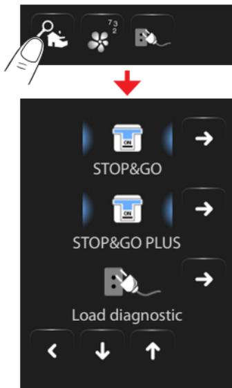
The status of each device will be displayed. Touch the
