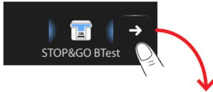
Enter the STOP&GO BTest details page to enable or disable the self-test function, by touching the **T** icon.
