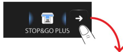
Enter the detail page of the STOP&GO PLUS device to force arming if any problems are shown by the status of the STOP&GO device itself.
