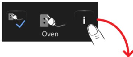
Access the load information page to display the current consumption. Use the
