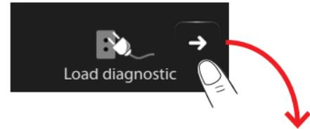
Access the Load diagnostic page to display the load status
