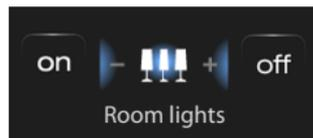
Use the – and + icons for the adjustment; the brightness of the light is not shown graphically.
