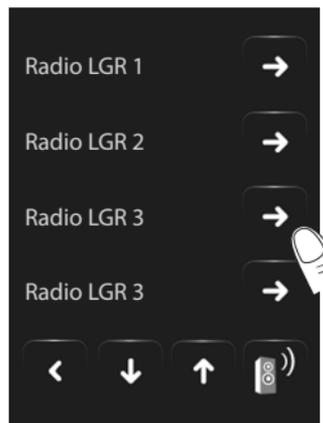
Select **→** on the display to load a new page for the display of all radio channels previously saved using the TouchScreenConfig software.
