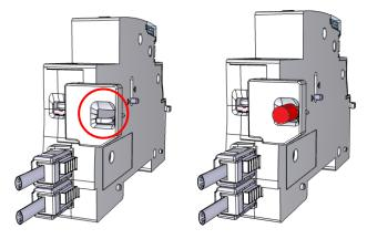
. Tool required to break the pre-fracture: flat screwdriver 2,5 mm . The port accepts the passage of 1 x 1,5 mm² cable with or without ferrule
