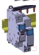
3. Pull the device downward in order to release it completely from the prongs of the busbar
