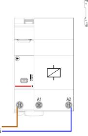
. Association with Contactor CX<sup>3</sup>, 1 DIN module width without handle (e.g. cat. no 4 125 05)
