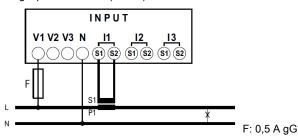
. 3 wires three-phase network, 3 sensors (3-3E):
