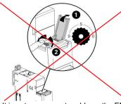
. It is not necessary to address the EMS CX<sup>3</sup> modules. The track wheel must be left in default position "0".
