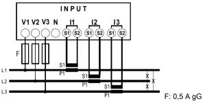
. 4 wires three-phase network, 3 sensors (3N-3E):
