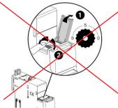
. It is not necessary to address the EMS CX<sup>3</sup> modules. The track wheel must be left in default position "0".
