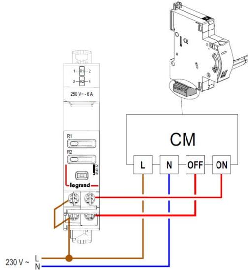
. Association with Motor Driven Control module DX<sup>3</sup> (cat. nos 4 062 90/91/92) with ON/OFF cyclic command
