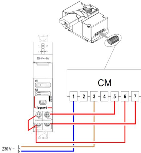
. Association with Motor Driven Control module DMX<sup>3</sup> 1600 (cat. nos 0 281 20/21/23) or Motor Driven Control module DMX<sup>3</sup> 2500/4000/6300 (cat. nos 0 288 34/35/37) with ON/OFF separated commands.
