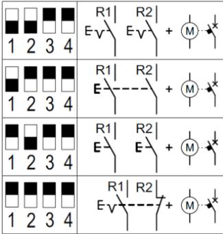
EMS CX<sup>3</sup> device associated with Latching relays or Contactors
