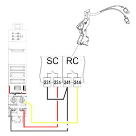
. Association with an electro-mechanical Signalling contact for DPX<sup>3</sup> or DMX<sup>3</sup> draw-out version (e.g. Cat. no 0 288 13 for DMX<sup>3</sup> / 0 265 74 for DPX<sup>3</sup>) or other brands auxiliaries.
