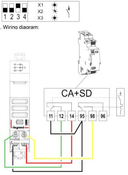
. Association with an electro-mechanical DPX<sup>3</sup> auxiliary contact (Cat. no 4 210 11) and DPX<sup>3</sup> fault contact (Cat. no 4 210 11) or other brands contact/fault auxiliaries.
