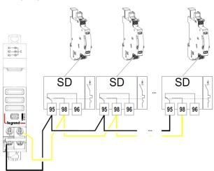
For DPX<sup>3</sup> fault contact auxiliaries use terminals 51 (instead of 95) and 54 (instead of 98) of the cat. no 4 210 11
