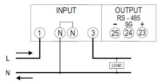
Protect the device with a circuit breaker with  $In \le 45 A$  (see the example)
