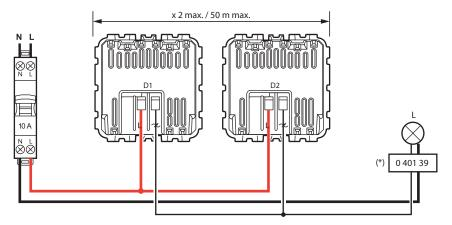
(\*) For some electronc loads, the installation of a compensator Cat. No. 0 401 39 is required.
