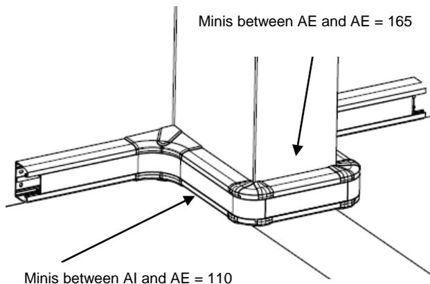
Mini dimension in mm to be respected allowing the installation of angle inter/exter: (in the case of a skirting of post for example)
