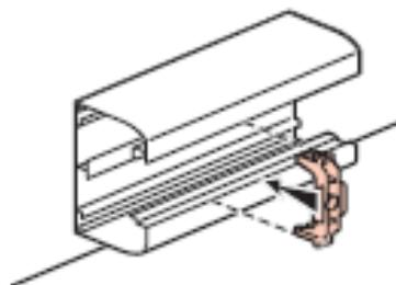
By removing the part of completion of the cover joint, that gives access simply the cover to withdraw it and facilitates the intervention in the compartment.
