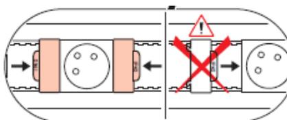
Installation principle for sockets for snap-on trunking :
