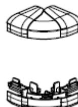
The external angles are delivered with 3 elements (ex: for trunking 2 compartment with partition junction)
