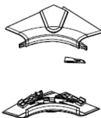
The internal angles are delivered with 3 elements (ex: for trunking 2 compartments with partition junction)
