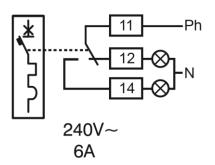
. (terminals marking on the  $2^{nd}$  CA are 21 / 22 / 24 when the selector of the reference 406 266 is in the "CA" position).
