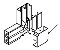
Positioning of the trunking to the wall before clipsage of the flat angle
