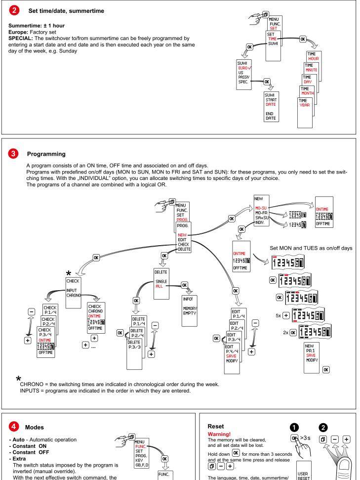
With the next effective switch command, the time switch resumes control of on/off switching.
